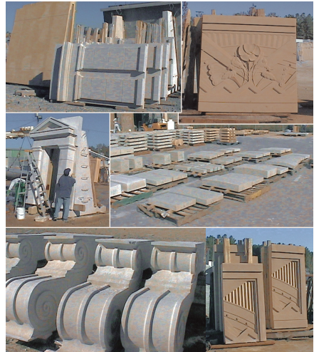
Pre-cast concrete sections comprise the exterior of the dome, ranging in size and weight from a briefcase to a small car.
